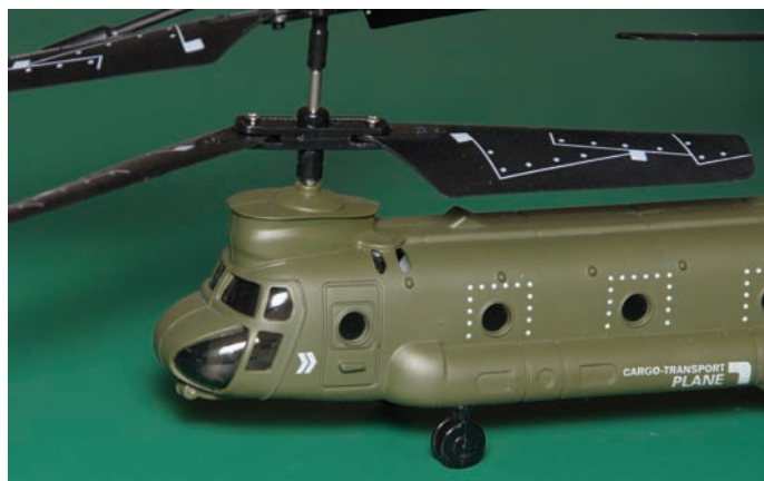
ABOVE: Nice detailing. The flexible rotors are an indoor safety feature intended to minimize damage to the heli and its surroundings!
