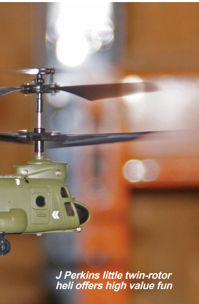
ABOVE: Nice detailing. The flexible rotors are an indoor safety feature intended to minimize damage to the heli and its surroundings!
