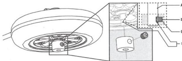
1. Loosely assemble an axle (A), screws (B), your choice of wheel and wheel collar (C) and set screw (D) on each retract strut. If needed, use nylon washers (E) as spacers to prevent the wheel from rubbing on the strut.
