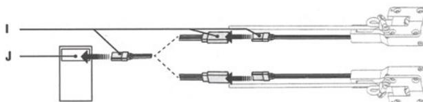
4. Connect the retracts to your receiver and extend the struts (if needed) to position the units in your aircraft. Mark the screw positions using the screw holes in the retract.
