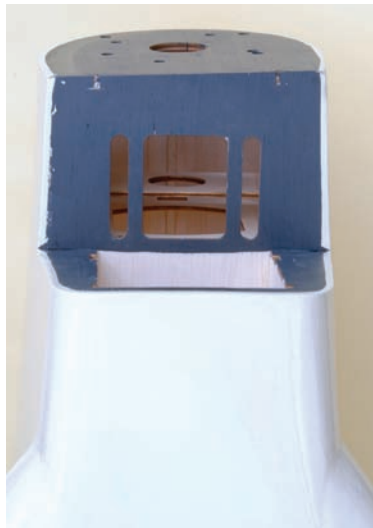
Built-in right thrust clearly shows up in this shot
