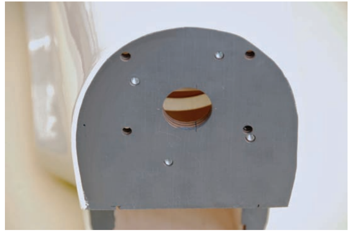
Mounting holes and fixings for both electric and I/C installations are incorporated; the weird mounting position for the I/C installation can be seen, but fortunately the thrust lines are marked on the former
