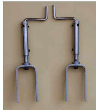
Substantial oleo legs and high quality spinner are typical of the quality of components in this kit
