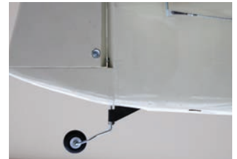
Distinctly un-scale tailwheel assembly
