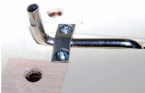
File flats onto the undercarriage torsion bars to make sure the legs don't twist and break the pretty fairing. If you can incorporate a little bit of toe-in ground handling will be improved also
