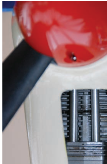
Plenty of cooling air can get directly onto the engine with this scale inlet
