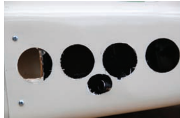
Cooling holes with additional exit hole for the 4-stroke silencer
