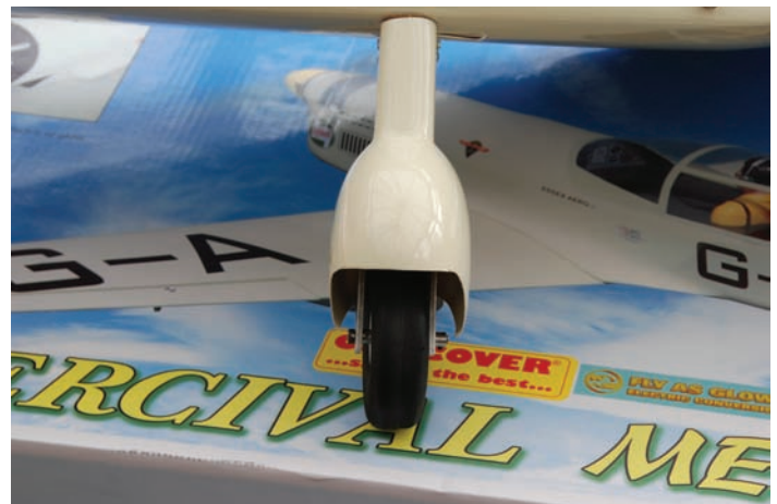
Completed undercarriage assembly with modified wheel fairing; note the slight toe-in on the wheel, also note that the fairing is set to ensure that the wheel can bounce up and down without interference
