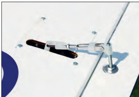
Mini units suit the laser-cut aileron mounts. In the best Seagull tradition the horns are threaded bolts.
