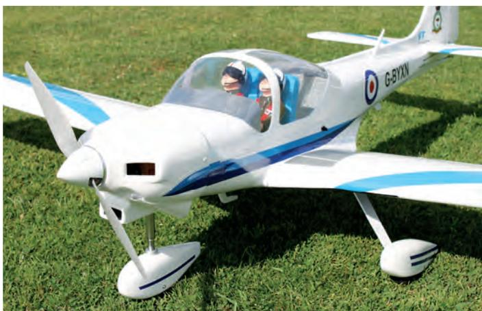
I toyed with opening up the lower vent but the top two provide plenty of cooling air to my ESC. As you can see, prop clearance isn't a problem.
