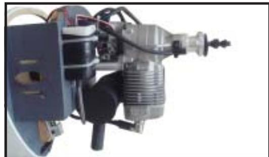
**!** *Blow through one of the lines to ensure the fuel lines have not become kinked inside the fuel tank compartment. Air should flow through easily.*
