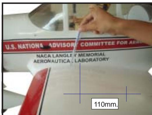
\*If possible, first attempt to balance the model by changing the position of the receiver battery and receiver. If you are unable to obtain good balance by doing so, then it will be necessary to add weight to the nose or tail to achieve the proper balance point.
