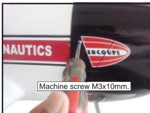
□ 3) Install the muffler and muffler extension onto the engine and make the cutout in the cowl for muffler clearance. Connect the fuel and pressure lines to the carburetor, muffler and fuel filler valve. Secure the cowl to fuselage using the M3x10mm screws.
