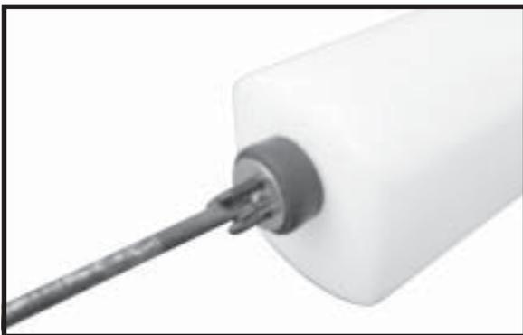
Attach the silicone fuel and pressure pipes to the tank. The lower pipe is the 'feed' and the upper two the 'pressure and fill'. The fill pipe is the next pipe.
