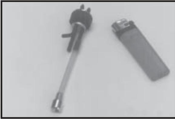
Carefully use a lighter or heat gun to permanently set the angle of the vent tube.
