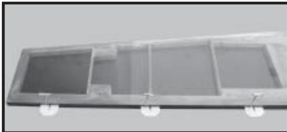
□ 3) Slide the elevator on the horizontal stabilizer panel until there is only a slight gap. The hinge is now centered on the horizontal stabilizer panel and elevator. Remove the T-pins and snug the elevator against the horizontal stabilizer panel. A gap of 1/64” or less should be maintained between the horizontal stabilizer panel and elevator.
