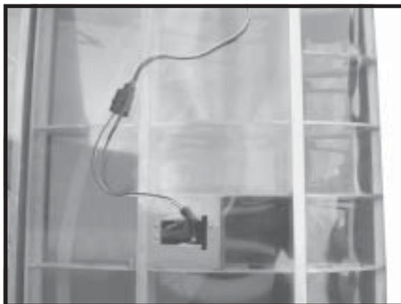
Attach a 12 inch servo lead to the aileron servo. Attach the string to the servo lead and carefully thread it through the wing. Once you have thread the lead through the wing, remove the string so it can use for the other servo lead. Tape the servo lead to the wing to prevent it from falling back into the wing.
