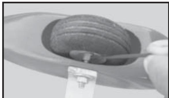
□ 4) A drop of C/A glue on the wheel collar screws will help keep them from coming loose during operation. Repeat the process for the other wheel.
