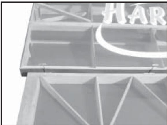
□ 4) Deflect the aileron and completely saturate each hinge with thin C/A glue. The ailerons front surface should lightly contact the wing during this procedure. Ideally, when the hinges are glued in place, a 1/64" gap or less will be maintained throughout the length of the aileron to the wing panel hinge line.
