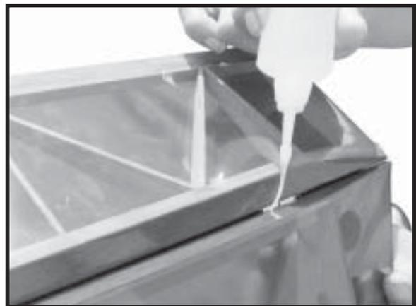
□ 6) Using C/A remover/debonder and a paper towel, remove any excess C/A glue that may have accumulated on the wing or in the aileron hinge area.
