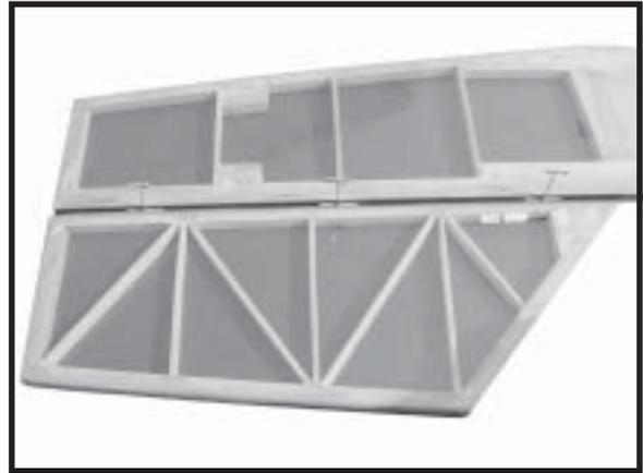
□ 4) Deflect the elevator and completely saturate each hinge with thin C/A glue. The elevators front surface should lightly contact the horizontal stabilizer during this procedure. Ideally, when the hinges are glued in place, a 1/64” gap or less will be maintained throughout the length of the elevator to the horizontal stabilizer panel hinge line.
