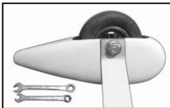
□ 4) A drop of C/A glue on the wheel collar screws will help keep them from coming loose during operation.
