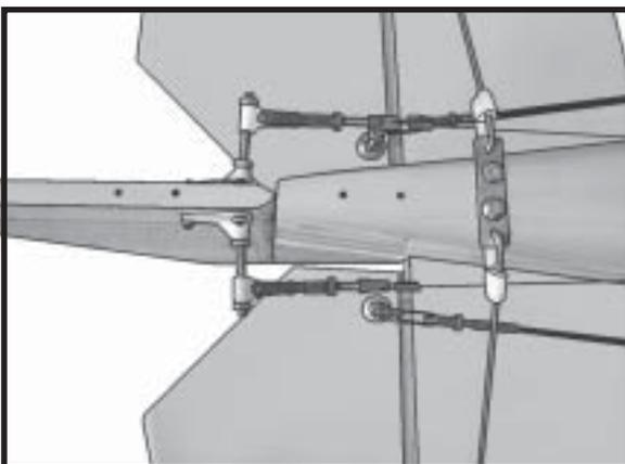
□ 4) Secure the tail wheel bracket in place using two 3x25mm wood screws. Be careful not to overtighten the screws.
