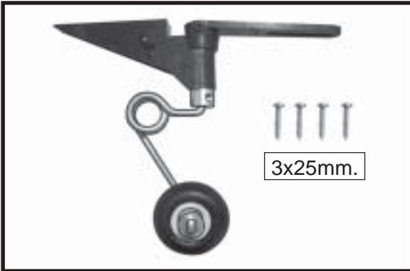
□ 2) Set the tail wheel assembly in place. The pivot point of the tail wheel wire should be even with the rudder hinge line and the tail wheel bracket should be on the plywood plate.
