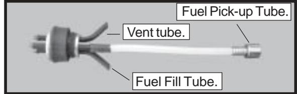
Carefully use a lighter or heat gun to permanently set the angle of the vent tube.
