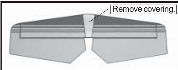
**!** *When cutting through the covering to remove it, cut with only enough pressure to only cut through the covering itself. Cutting into the balsa structure may weaken it.*
