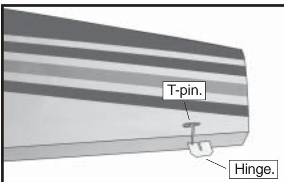
□ 3) Slide the wing panel on the aileron until there is only a slight gap. The hinge is now centered on the wing panel and aileron. Remove the T-pins and snug the aileron against the wing panel. A gap of 1/64" or less should be maintained between the wing panel and aileron.
