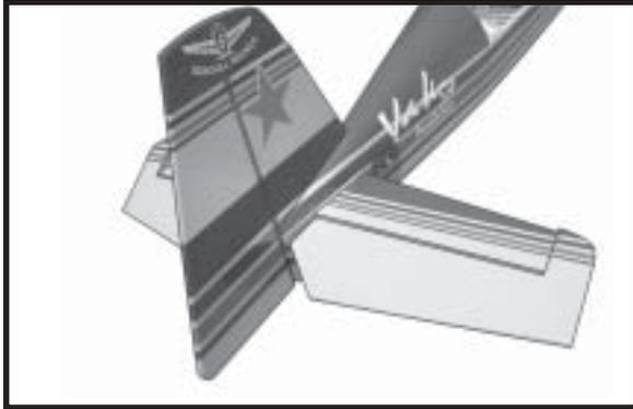
□ 3) While holding the vertical stabilizer firmly in place, use a pen and draw a line on each side of the vertical stabilizer where it meets the top of the fuselage.
