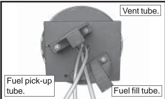
**!** *Blow through one of the lines to ensure the fuel lines have not become kinked inside the fuel tank compartment. Air should flow through easily.*
