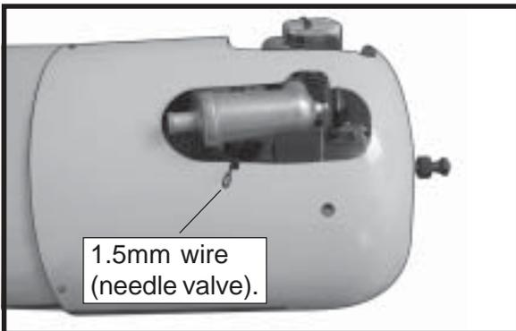
□ 3) Install the muffler and muffler extension onto the engine and make the cutout in the cowl for muffler clearance. Connect the fuel and pressure lines to the carburetor, muffler and fuel filler valve. Secure the cowl to fuselage using the 3mmx10mm screws (4).
