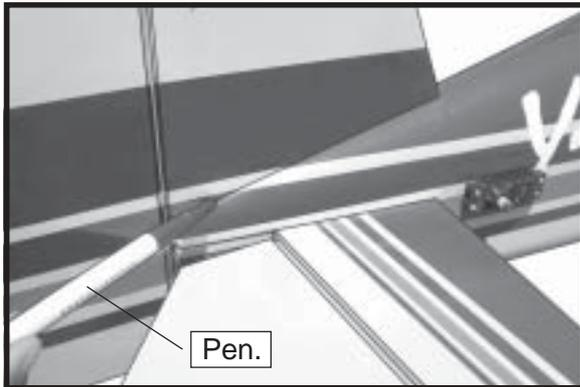
□ 4) Remove the stabilizer. Using a modeling knife, remove the covering from below the lines you drew.
