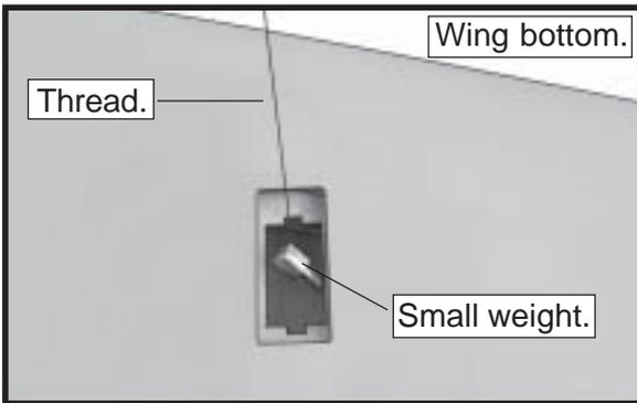
Attach the string to the servo lead and carefully thread it through the wing. Once you have threaded the lead through the wing, remove the string so it can be used for the other servo lead. Tape the servo lead to the wing to prevent it from falling back into the wing.
