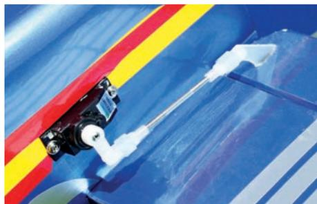
I slipped some ParkZone micros in at the tail, although some trimming was required for a good fit.
