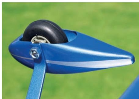
Whilst the glass fibre spats are strong enough, the small wheels will only cope with smoother take-off surfaces.
