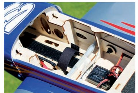
With elevator and rudder servos sited at the tail, there's plenty of room here for the battery and Rx.
