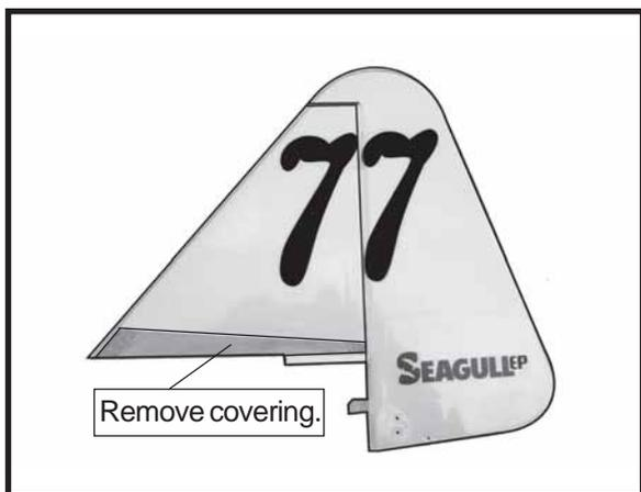
□ 5) Slide the vertical stabilizer back in place. Using a triangle, check to ensure that the vertical stabilizer is aligned 90° to the horizontal stabilizer.
