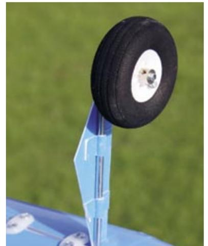
plastic saddle clamps that straddle the wire legs from behind. With this each undercarriage leg is clamped into a wing-mounted block using the conventional saddles provided in the hardware pack. The tail wheel is soon fitted, a fairly standard unit that's surprisingly tall, sitting the tail quite a way from the ground. As is the established norm these days, all of the Texan's control surfaces are attached with Mylar hinges, these being secured with a wick of cyano.
