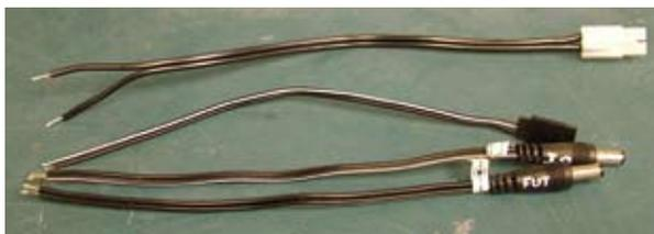
The Vector NX81 charger is supplied with four alternative charging leads. These are clamped into the output block as needed. It is wise to colour code the positive cables with a blob of red paint to ensure correct connection into the charger output block.
