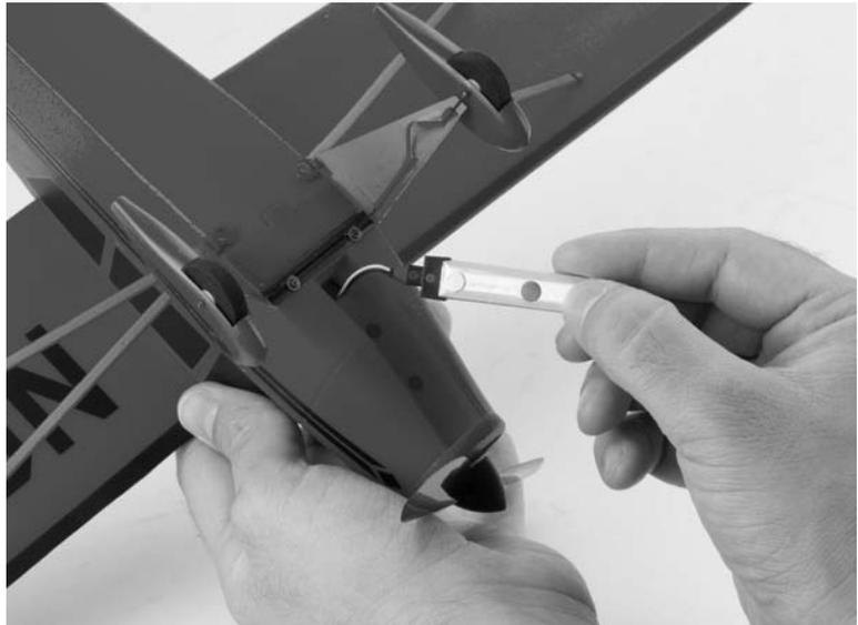
To remove the LiPo flight battery, lift it away from the magnets then disconnect it from the 3-in-1 control unit. **DO NOT** power off the transmitter until the LiPo flight battery is removed from the airplane and the 3-in-1 control unit is powered off. **REMEMBER: The transmitter is always on first and always off last!**
