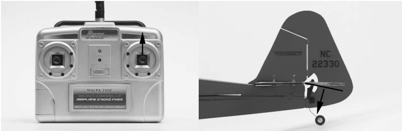
Pulling the stick backward/downward will raise the elevator and pitch the nose of the airplane upward to climb.
