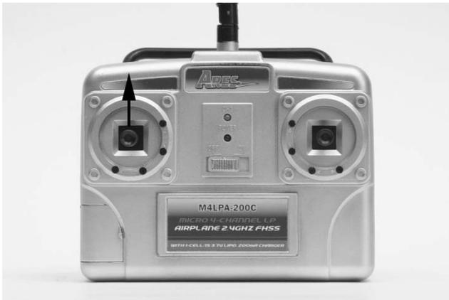
Moving the stick upward will increase the speed/RPM of the propeller. Increasing the speed of the propeller increases the speed of the model and also provides the thrust needed to climb/increase altitude.
