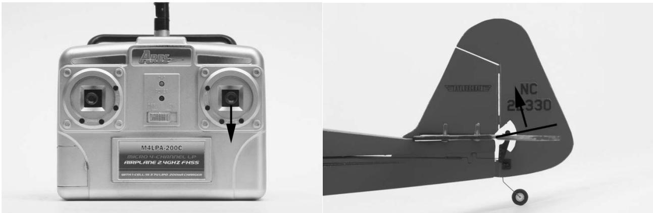
The elevator channel trim (the buttons located directly to the left of the right-hand stick) can be used to help keep the airplane from climbing or descending when in cruise flight and with no right-hand stick/elevator control input. For example if the airplane climbs when attempting to cruise and maintain a given altitude, add down elevator trim by pressing the top trim button until the airplane flies as level as possible and maintains the desired altitude at cruise speed.
