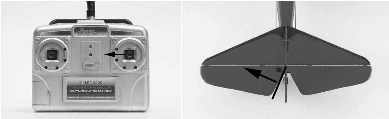
Moving the stick to the right will move the rudder to the right. This will roll/turn the airplane to the right.
