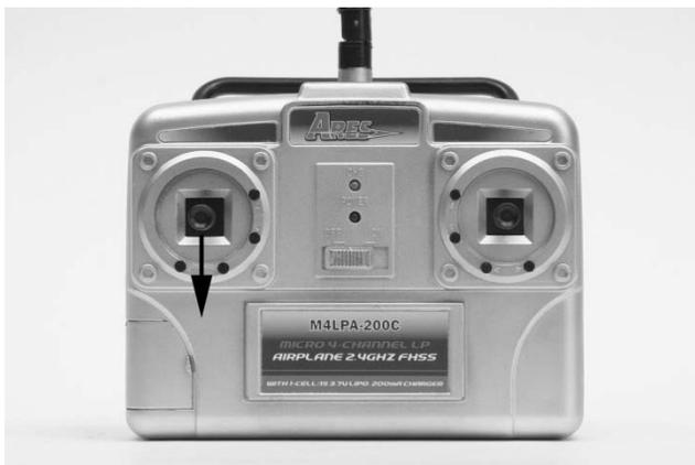
Decreasing the speed/RPM of the propeller by lowering the left-hand stick will decrease the speed of the model and reduce thrust making it possible to descend/decrease altitude.
