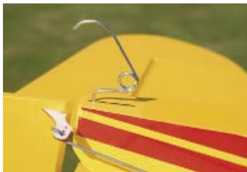
*I used GWS mini servos all round. The swing keepers are mine so do note that if you go this route your wire bending needs to be accurate!*
