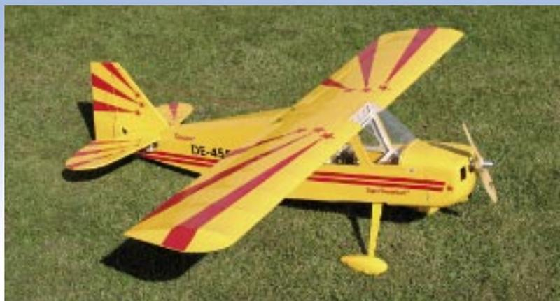
Landings are a straight-forward undertaking, indeed I was surprised how well the small wheels and spats coped with short grass. That said, I'm sure normal length grass will induce a nose-over flourish at some stage in the process. The model will float down perfectly on a calm day but needs some throttle management to bring her in on windy ones, although this would apply to most models of
