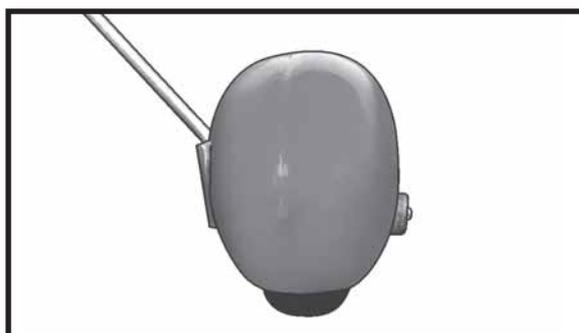
A drop of C/A glue on the wheel collar screws will help keep them from coming loose during operation.
