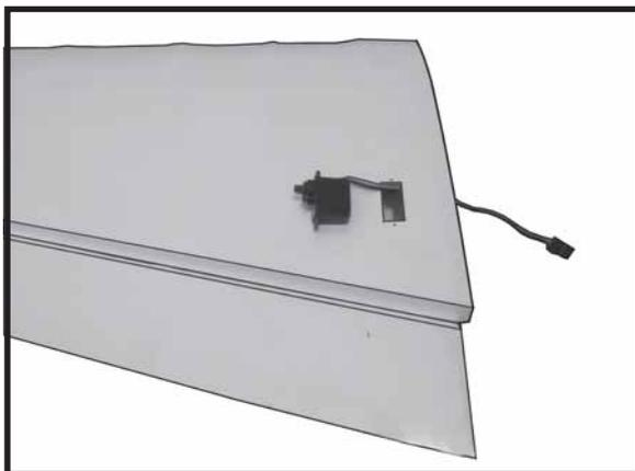
Secure the servos with the screws provided with your radio system.
