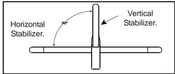
□ 6) When you are sure that everything is aligned correctly, mix up a generous amount of 30 Minute Epoxy. Apply a thin layer to the mounting slot in the top of the fuselage and to the sides and bottom of the vertical stabilizer mounting area. Apply epoxy to the bottom and top edges of the filler block and to the lower hinge also.
