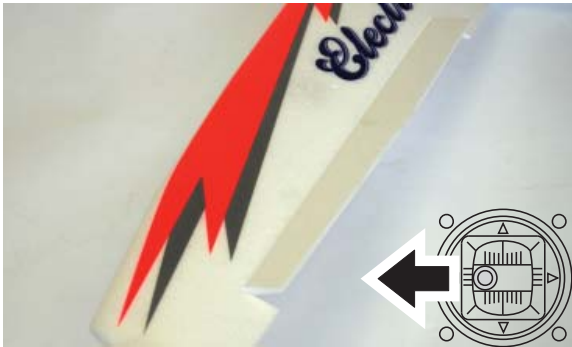
Left Aileron (up)
