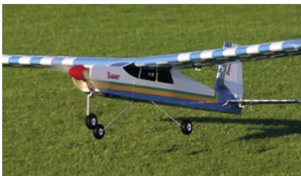
exactly 5 lbs, although the 600+ square inches of wing still make the E-Pioneer a bit of a floater.
