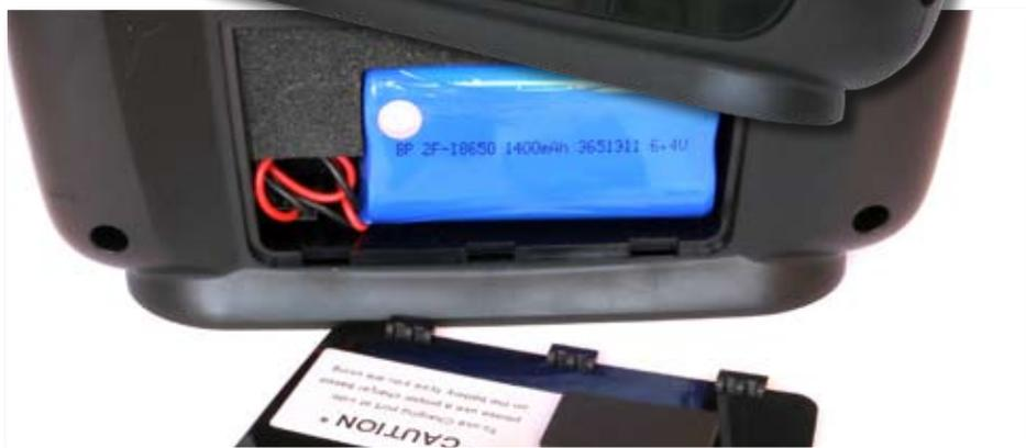
*The 1400 mAh LiFe battery pack is accessed through a panel at the rear of the transmitter*
