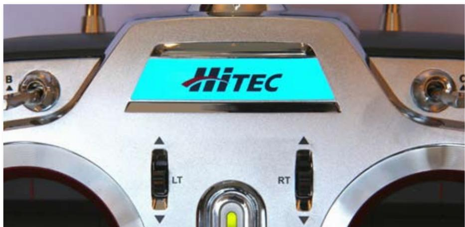
*The top trim switches, marked LT and RT, are for additional channels*
