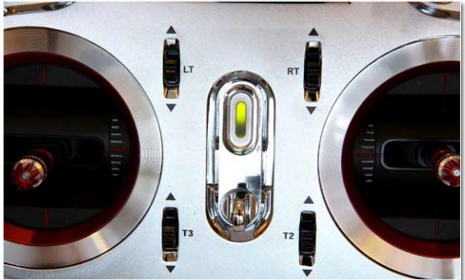
Flash 8 features the usual digital trims. Push the power button and the Flash 8 wakes up instantly
