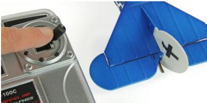
Pull the elevator stick back and check that the elevator moves in an upward direction. Push the elevator stick forward and check that the elevator moves in a downward direction.
