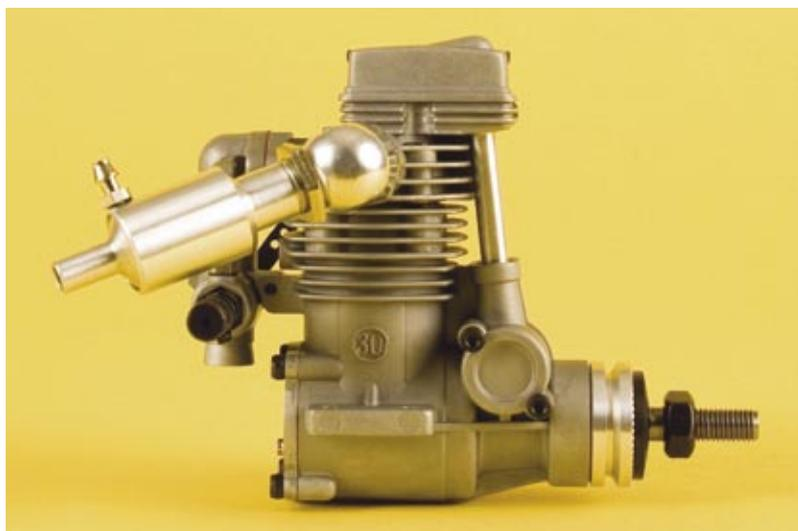
period! I have to take the engines to bits that drop into my reviewers cache, but the old adage 'if it ain't broke, don't fix it' certainly applies to model engines. Four-strokes have more bits and bobs whizzing around inside than two-strokes, and that all-essential valve timing must be noted during disassembly; incorrect reassembly will prevent the engine from running and the valves could tangle, resulting in severe damage.
