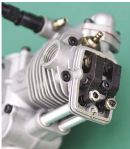
*The twin rockers that operate the two perpendicular, spring-loaded, overhead valves.*
