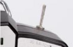
The Twister CP V2.1 transmitter features an idle up switch. This is for use when flying outdoors and for performing aerobatic manoeuvres.
