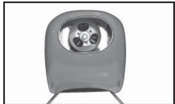
□ 2) Slide the fiberglass cowl over the engine and line up the back edge of the cowl with the marks you made on the fuselage then trim and cut.
